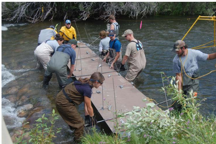
A crew installs a PIT tag antenna in the Lemhi River in Idaho, an intensively monitored watershed.
